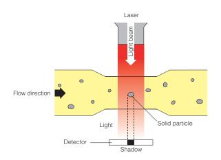
The contamination level identifies the quantity and dimensions of solid particles present into the hydraulic fluid. It is classified according to the European standard ISO 4406/1999, while for North America it is classified by SAE AS 4059 or NAS 1638 standards.
